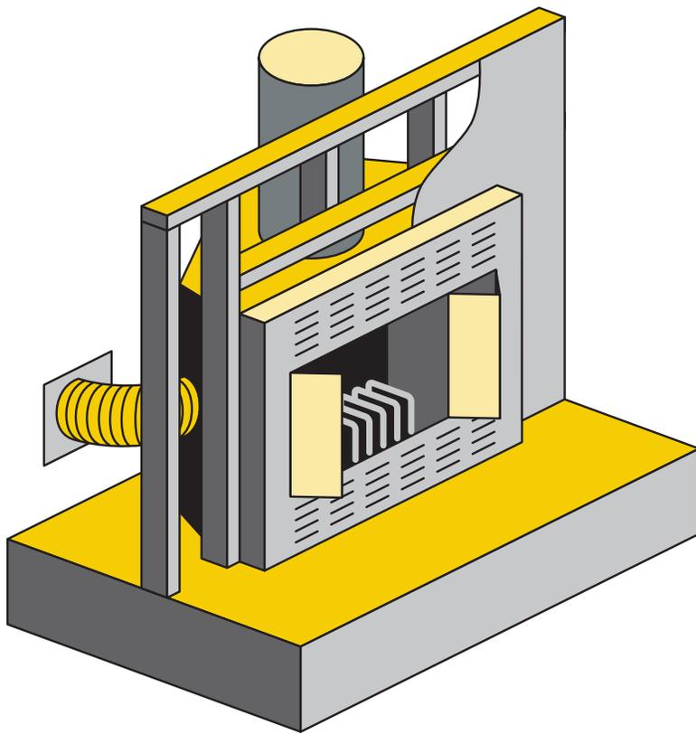
*Keep your fireplace damper closed unless a fire is going. Leaving the damper open is like throwing open a 48-inch window. The damper should be well sealed. It's best to cover the firebox opening with metal or glass doors, which will restrict the amount of heated air drawn from the house. ◀*
