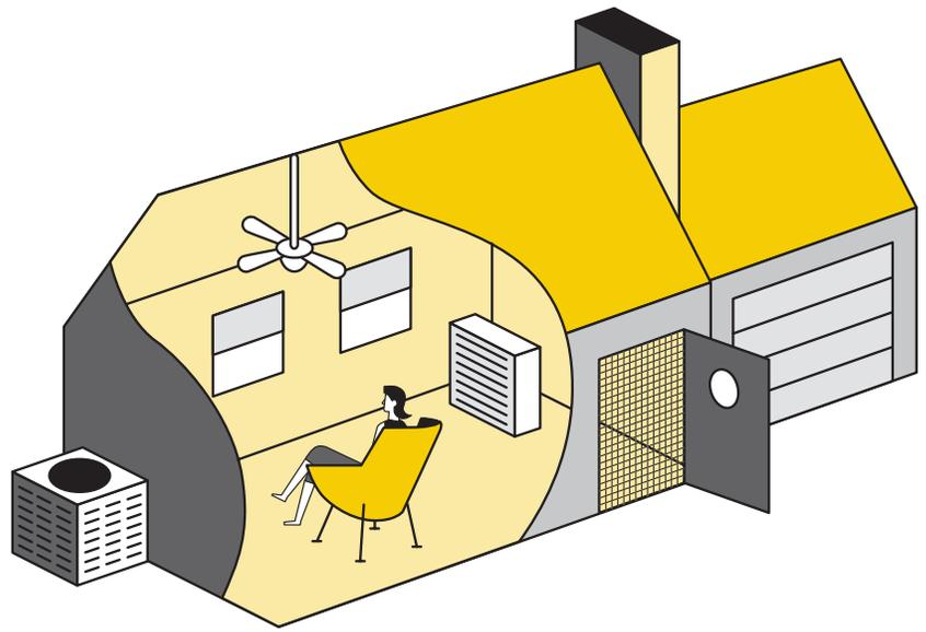
In spring and fall, when it's not particularly hot or cold, a whole house fan can be an excellent alternative to your central system. Installed in the ceiling, a whole house fan draws outdoor air inside to cool the house.
